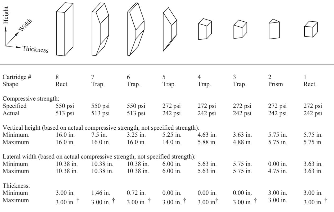
† Maximum thickness after cartridge pre-crushing. Material thickness prior to pre-crushing was 3.25 in.
