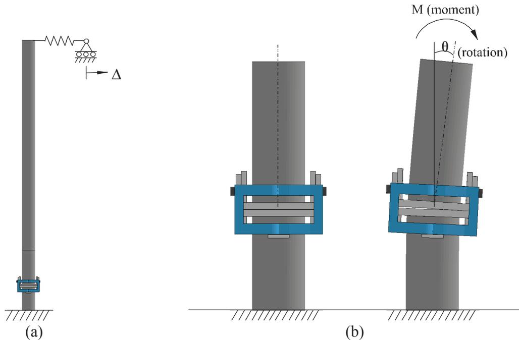
Figure 6.3 Finite element pushover analysis:
