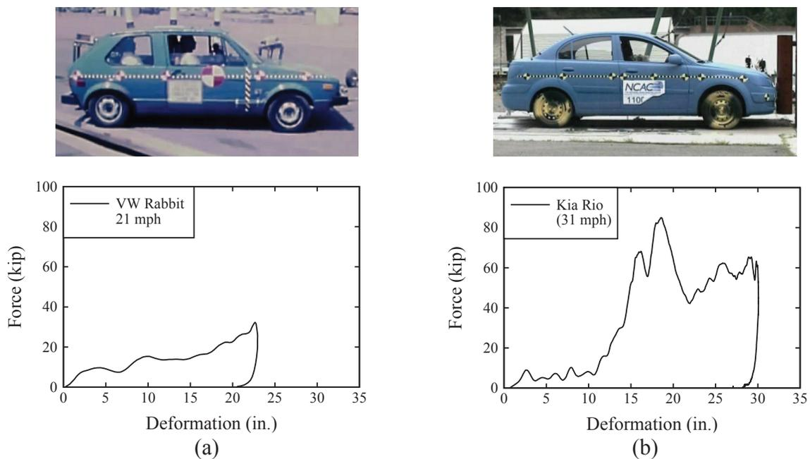
Figure 3.1 Production vehicles and force-deformation data:
