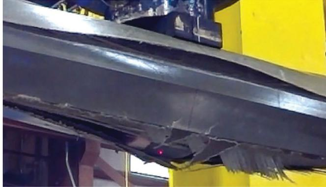
Figure 4.9 Detailed view of FRP condition after failure
