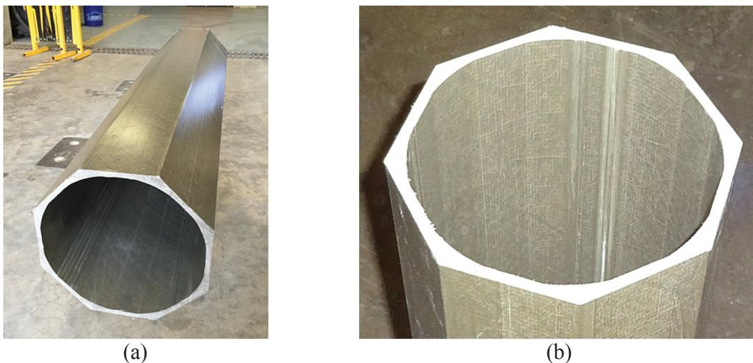
Figure 4.1 Octagonal CP076 FRP power pole manufactured by Creative Pultrusions:
