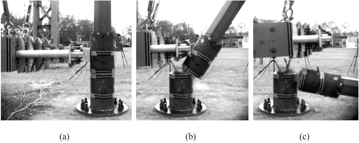
Figure 5.6 High speed video frames from impact testing of shear collar hybrid connection:
