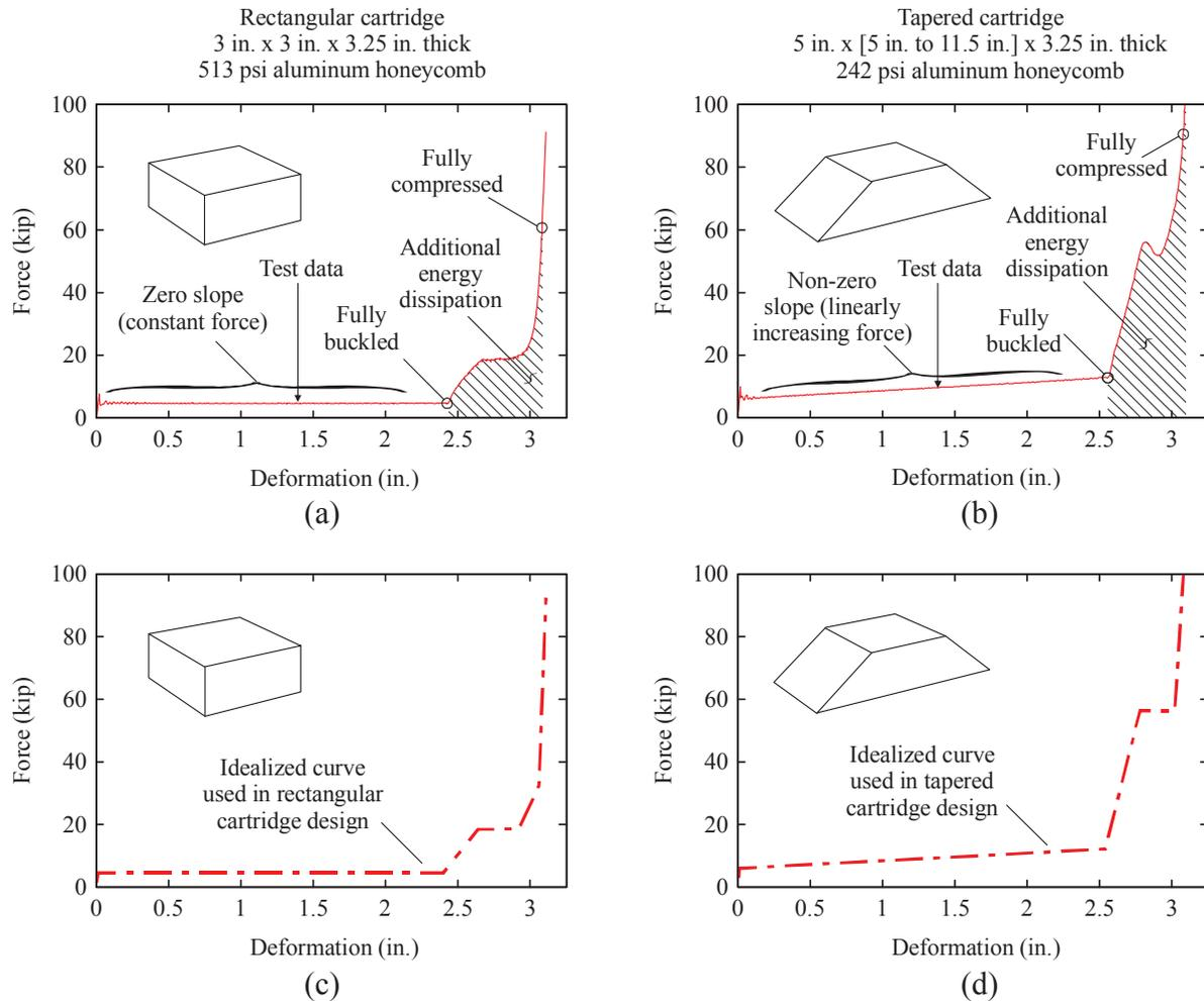
Figure 3.6 Compression test data and idealizations used in cartridge design:
