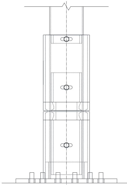
Figure 5.2 Shear collar hybrid breakaway system concept
