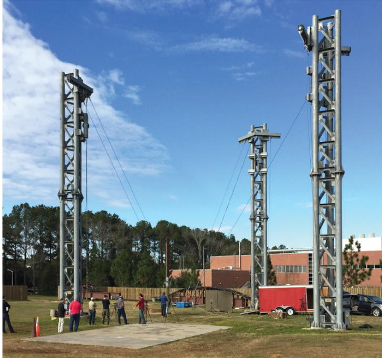
Figure 6.6 Impact pendulum at FDOT Structures Research Center (Tallahassee, FL)
