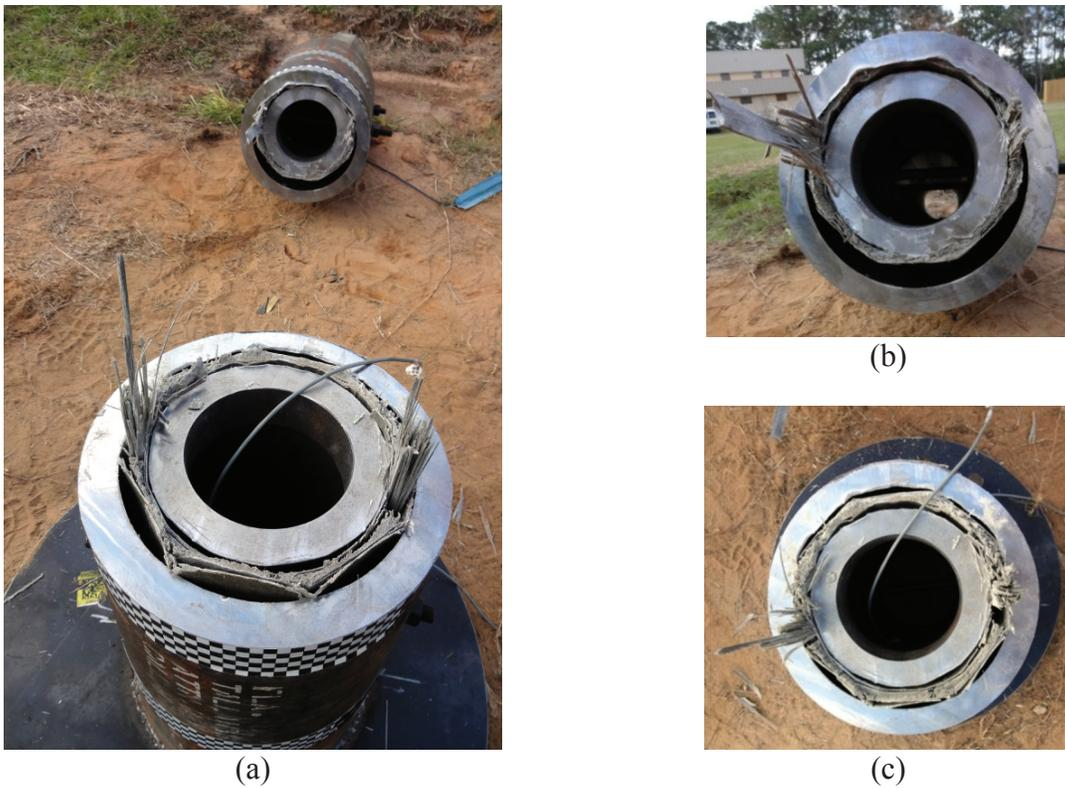
Figure 5.7 Condition of FRP post and cutting edges after impact test:
