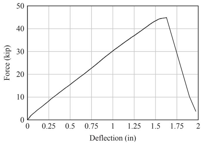
Figure 4.8 Static flexural test results
