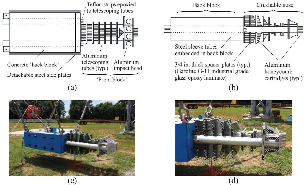
Figure 3.9 Crushable nose 1100C surrogate vehicle:
