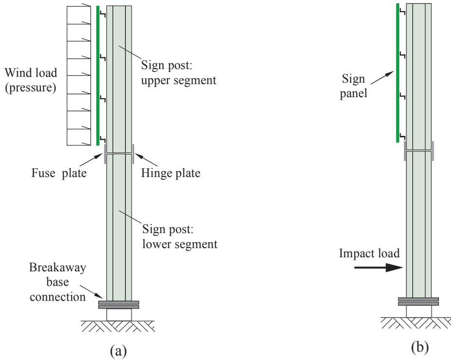
Figure 1.1 Design loading conditions on a roadside sign structure:
