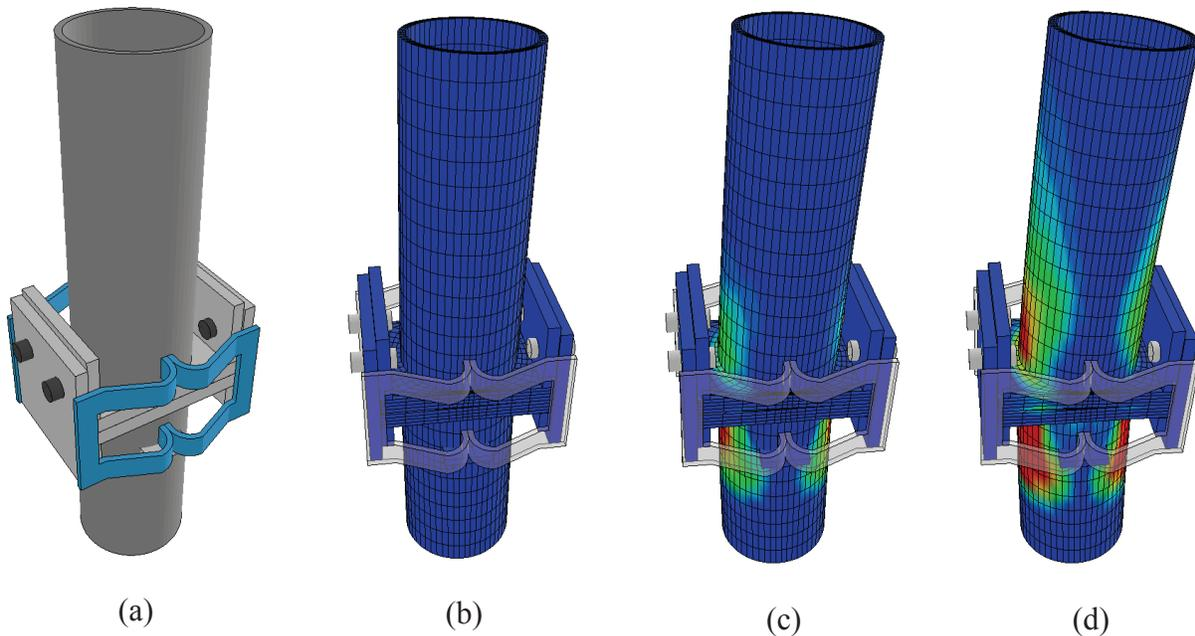
Figure 6.4 Plastic strains from pushover analysis of moment collar with HSS stem:
