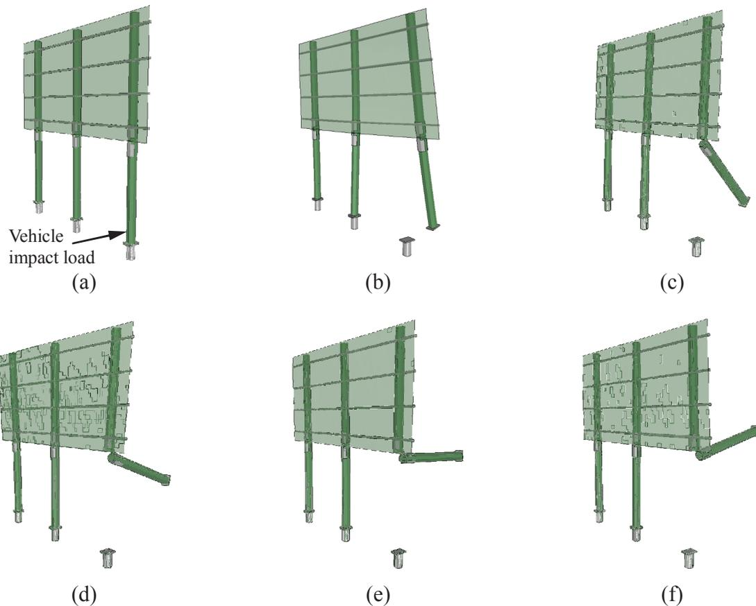
Figure 1.3 Intended system behavior of a three-post sign structure:
