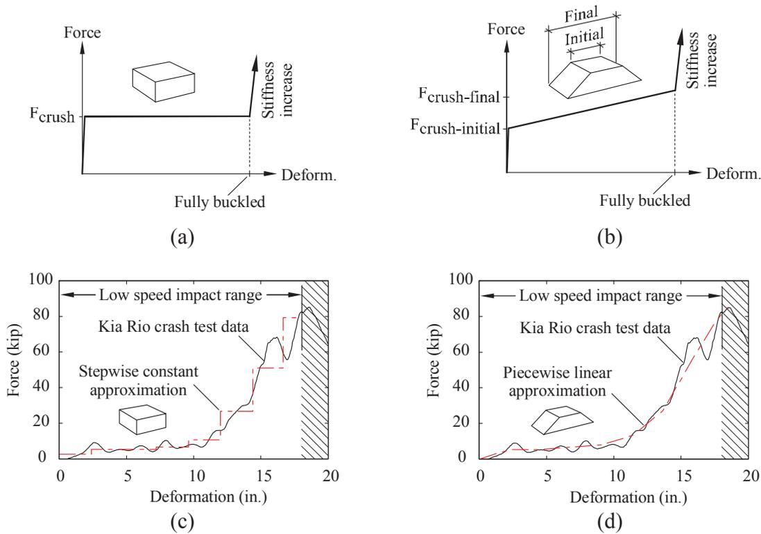
Figure 3.3 Simplified description of production vehicle force-deformation curve approximation:
