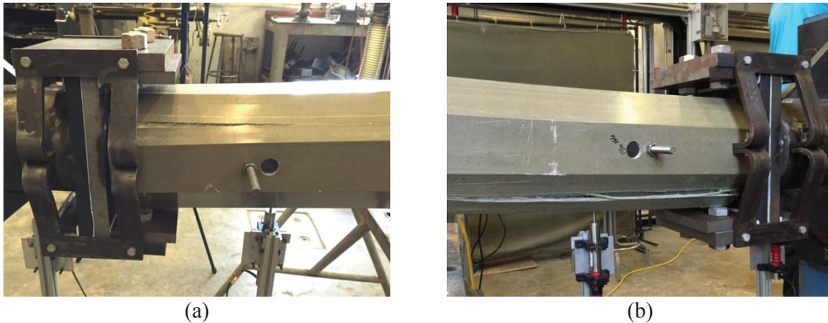
Figure 6.23 Longitudinal failure lines:
