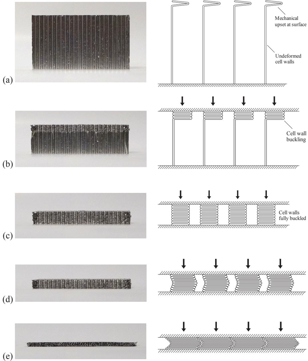
Figure 3.5 Stages of aluminum honeycomb compression behavior:
