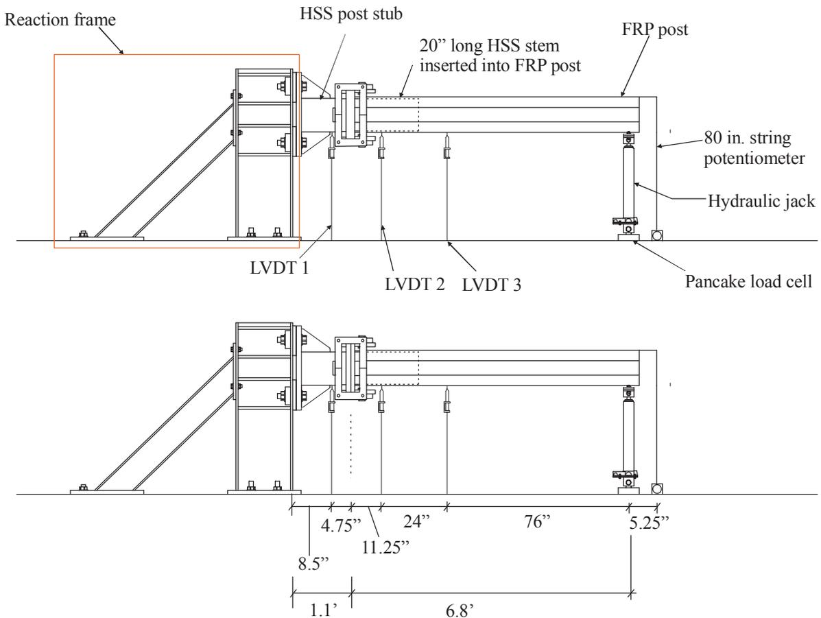
Figure 6.20 Schematic diagrams of static flexural test setup
