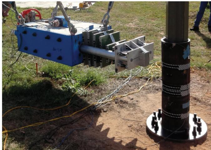
Figure 5.5 Impact test for shear collar connection concept
